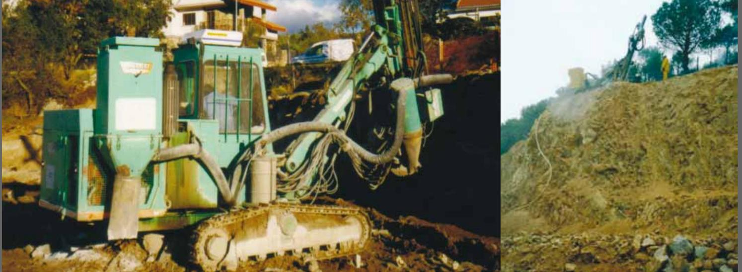
**Voladuras y Demoliciones** performs all types of rock fragmentation, from the perforation and blasting procedure to the crushing and its classification for the production of artificial crushed aggregates.
