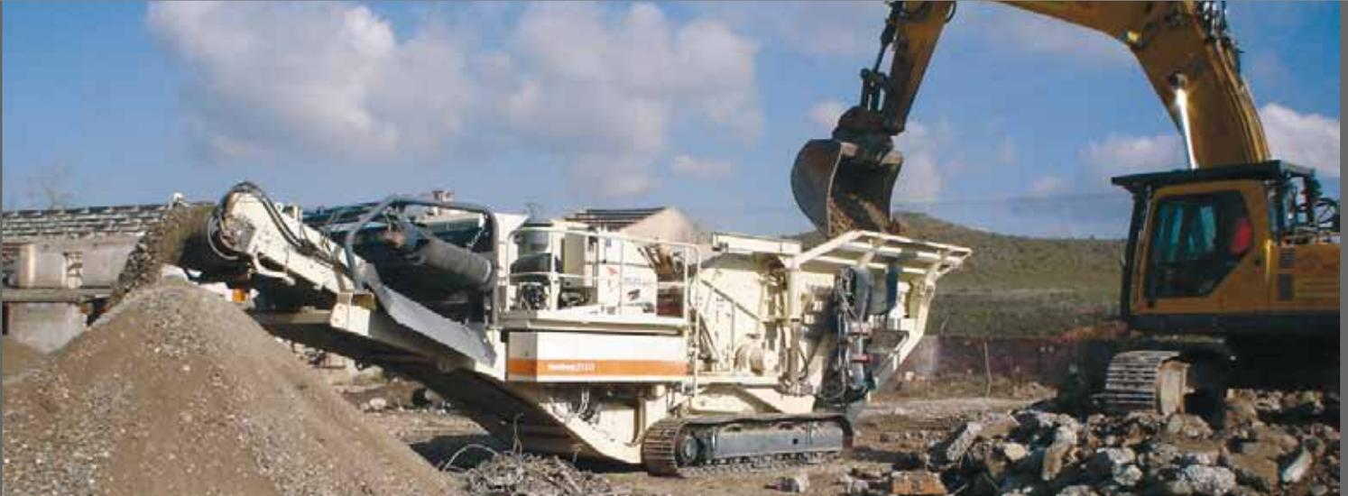
**Voladuras y Demoliciones** performs the recycling of stone materials of the demolition (concrete, ceramics and masonry) or from the excavations using portable groups of crushing machines and classification of track-mounted screening plant.
